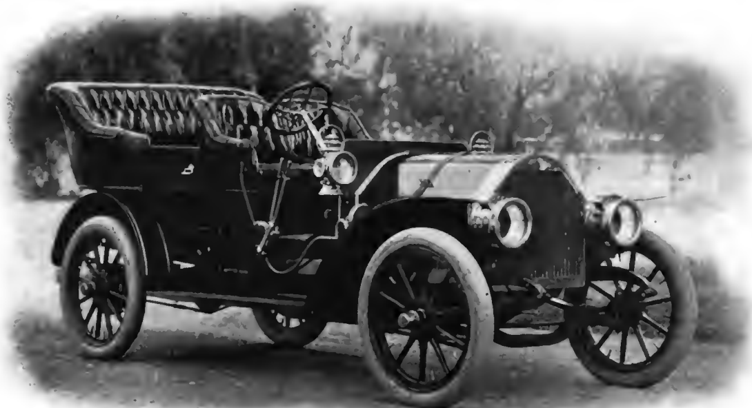
THOMAS "FORTY," 40-H.P., 4 CYLINDERS, PRICE $2,750. E. R. Thomas Detroit Co., Detroit, Mich.
